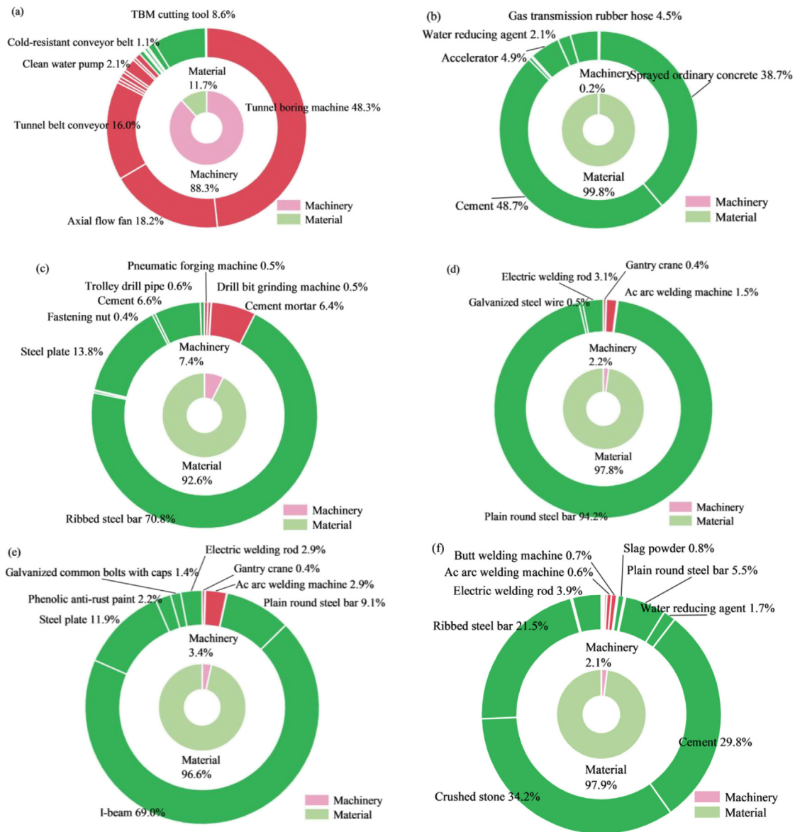
Fig. 9. Actual carbon emission characteristics of the tunnel. (a) CE_{exc} , (b) CE_{con,support} , (c) CE_{bo,support} , (d) CE_{rfm,support} , (e) CE_{sf,support} , and (f) CE_{lining} .
