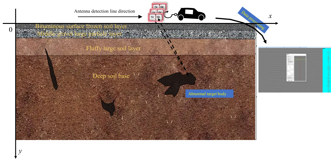
Fig. 6. Ground-penetrating radar detection principle diagram.
