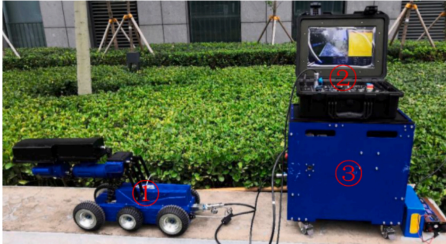
Fig. 8. CCTV-detecting device consists of a tractor (mark 1), a control system (mark 2), and a cable tray (mark 3) (Ma et al., 2021; reproduced with permission, courtesy of Elsevier).
