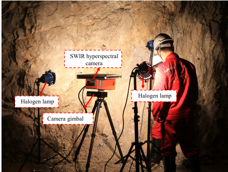
Fig. 15. In-situ hyperspectral image acquisition of the tunnel.
