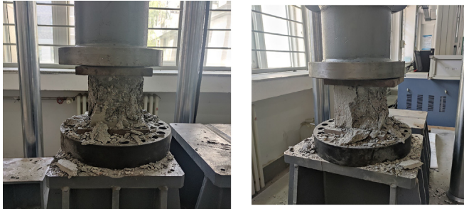
Fig. 3. Concrete cube compressive strength test.
