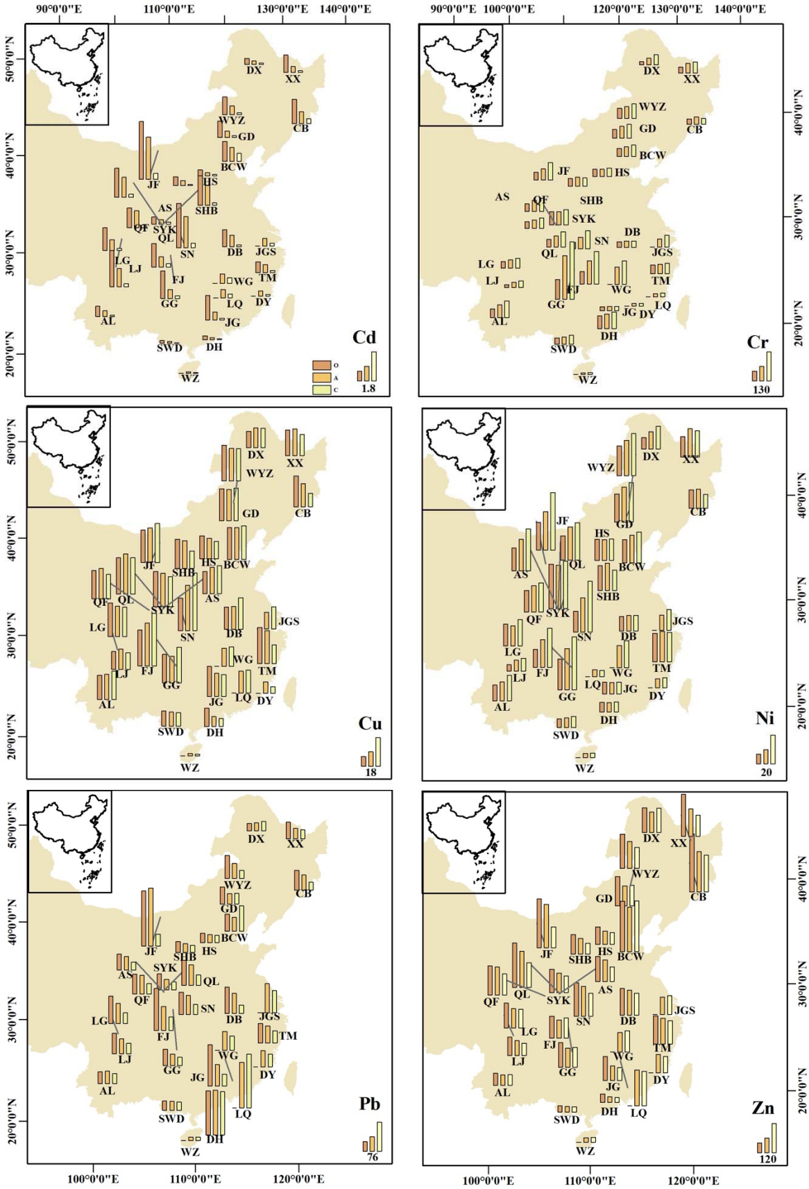
Figure S1 The spatial distribution of trace metals (mean, mg/kg) in the mountain soils across China. The figure was mapped by the R 4.0.3 software.
