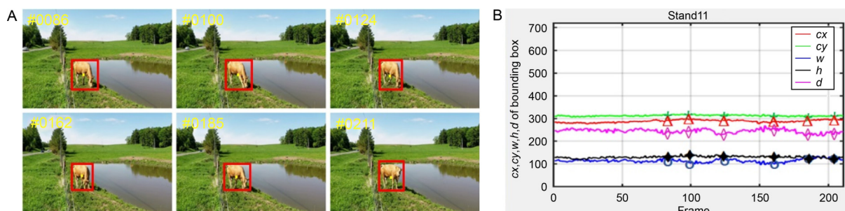
Figure 3. The action of standing about video (stand11). (A) Six target rectangles and their centres; (B) The five curves of state parameters.
