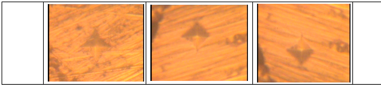
Figure 5. Micro-indentation images showing different measurements of microhardness of the composite samples.
