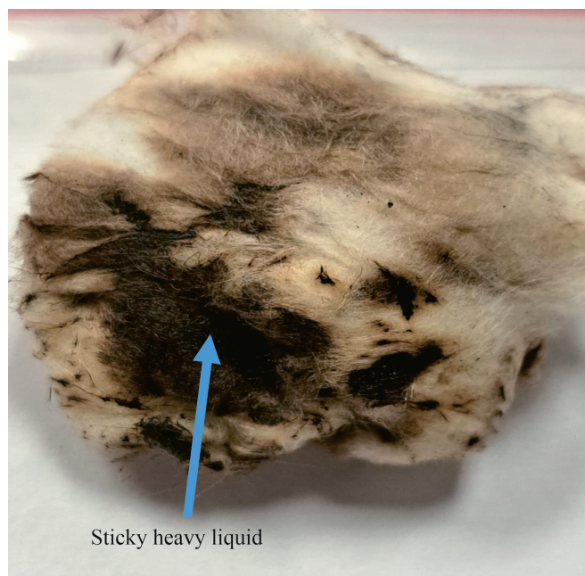
Fig. 7. Sticky heavy liquid deposited on top of quartz wool at low pyrolysis temperatures.
