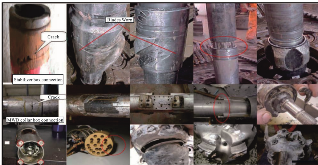
Fig. 3. Downhole tool damage caused by stick-slip [14].
