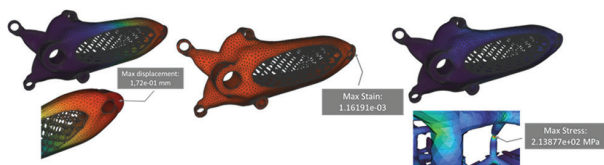
Figure 10. Results of the static test held in nTopology (1300 N)
