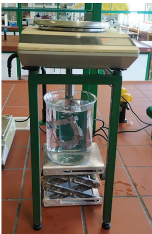
Figure 9. Archimedes test rig for buoyancy and density measure
