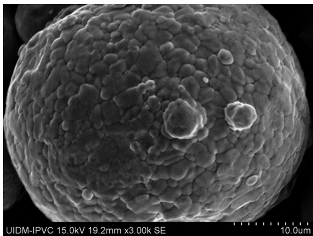
Figure 5. Scanning electron microscopy image at 3000 \times magnification of Tool Steel 1.2709-A LMF (TRUMPF) powder particle Abbreviation: SEM: Scanning electron microscopy
