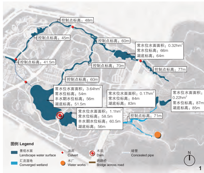
1. 烟台植物园水系统图 2. 建设中的烟台植物园：连接山地汇水区与湖区的道路涵洞桥。 3. 建设中的烟台植物园：设计将汇水冲积区保留的蓄水池和新建设的主湖区连接在一起。 1. Water system of Yantai Botanical Garden 2. Yantai Botanical Garden under construction: the road culvert bridge connects the mountain watersheds and the lake area. 3. Yantai Botanical Garden under construction: the reserved reservoir in the alluvial watersheds combined with the newly-built main lake.
