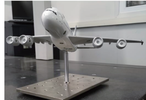
(b) Airplane model is stably supported at a certain elevation angle through a support rod
