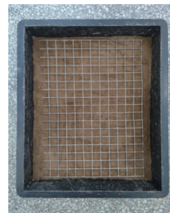
(b) Drainage net structure
