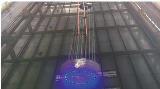
Fig. 1 Light source marker at docking station
