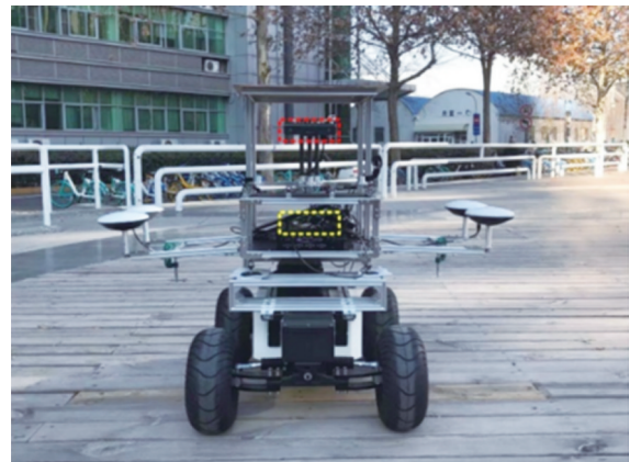
Fig. 8 Data collection platform for our experiments in large-scale outdoor scenes: A MYNTEYE-D1000-50 (red part) is used to capture images and IMU data, and a Novatel PwrPak7D-E1 (yellow part) is used to provide ground truth trajectories
