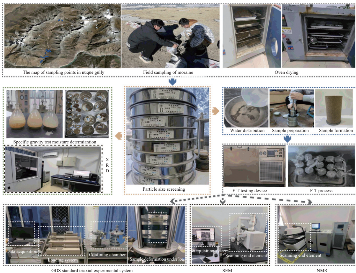
Fig. 2 The flowchart diagram of the experimental procedure
