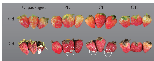
Fig. 9 Time-lapse photographs of strawberries sealed by different films
