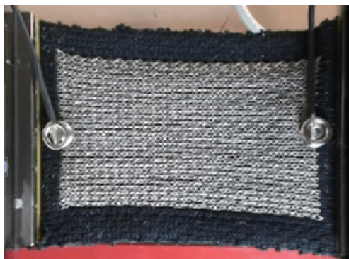
Fig. 3 Knitted fabric electrode [24]
