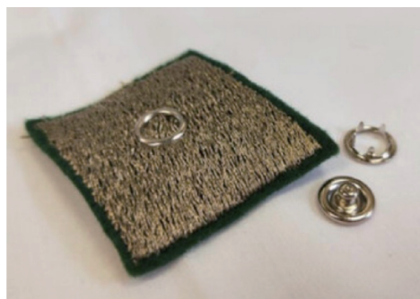
Fig. 4 Embroidered fabric electrode sample with snap fastener parts [28]
