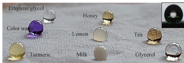
Fig. 6 Different droplet morphologies on cotton fabric after antifouling finishing [32] (Copyright 2019, Elsevier, all right reserved)
