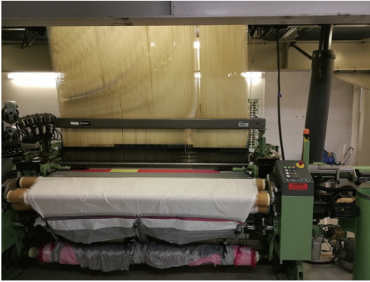
Fig. 3 POF textile weaving on Jacquard loom
