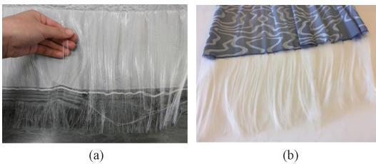
Fig. 11 POF floats: (a) before separated from selvage; (b) after separated from selvage
