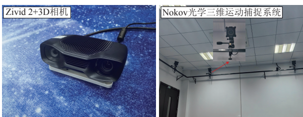
图 10 Zivid 2 + 3D相机及Nokov光学三维运动捕捉系统 Fig. 10 Zivid 2 + 3D camera and Nokov optical 3D motion capture system
