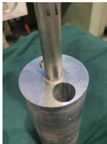
图8 热管/燃料钎焊样件 Fig. 8 Braze welding sample of heatpipe and fuel
