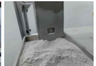
(c) 采样铲内样本脱落
