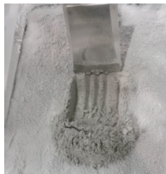
(c) 采样铲对月壤水冰采样
