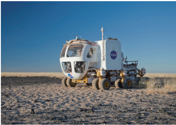
图 2 NASA设计的加压月球车 [14] Fig. 2 Pressurized lunar rover designed by NASA [14]
