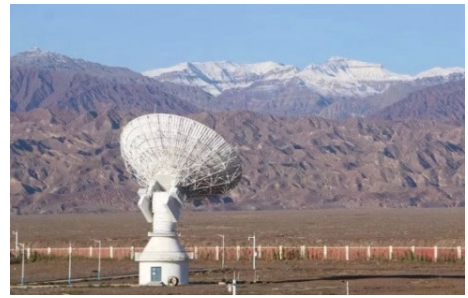
图13 搬迁至喀什深空站场区的18 m S/X双频段测控设备 Fig. 13 18 m S/X -band TT&C equipment relocated to Kashi deep space station site
