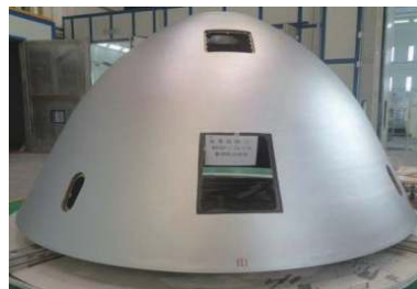
图8 低吸收比低发射率涂层 Fig. 8 Low absorption and low emission coating
