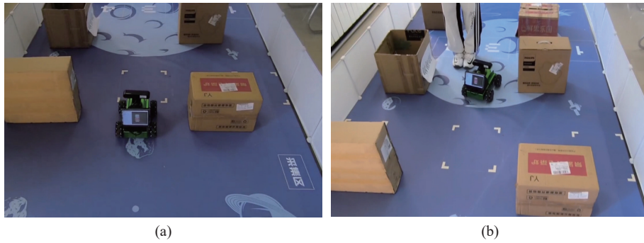
Fig. 10 Changes in the movement direction of the small car before and after dynamic obstacle avoidance: (a) movement direction of the small car before obstacle avoidance; (b) movement direction of the small car after obstacle avoidance
