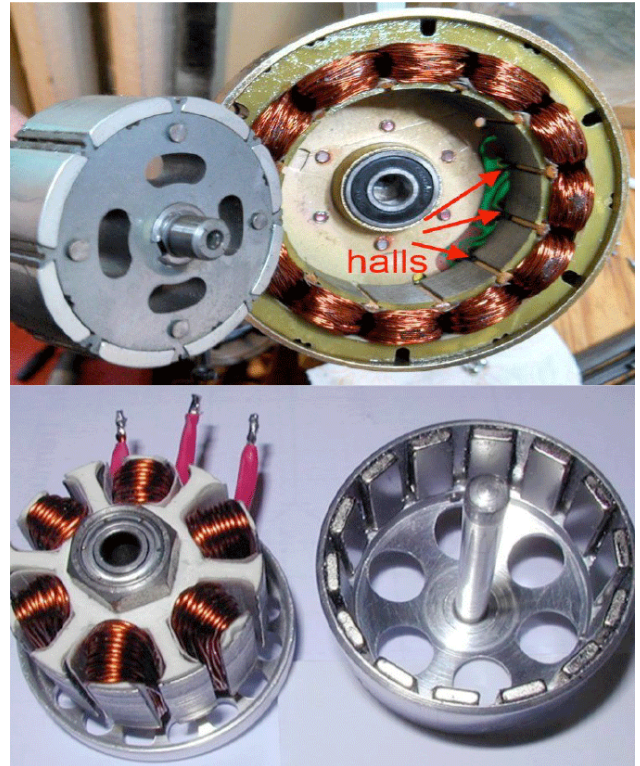
Figure 1. Schematic of a brushless direct current motor 25
