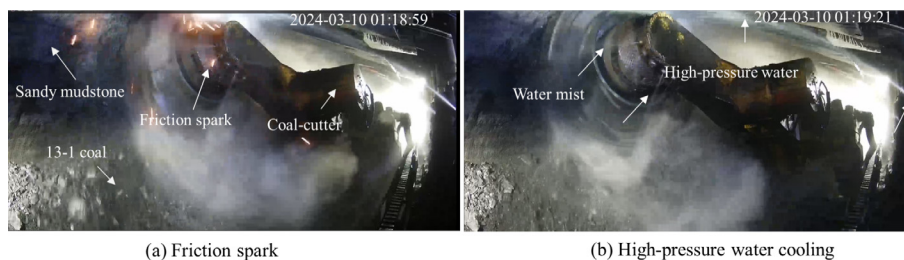
Fig. 21. High-pressure water injection to suppress frictional sparks between picks and rocks.
