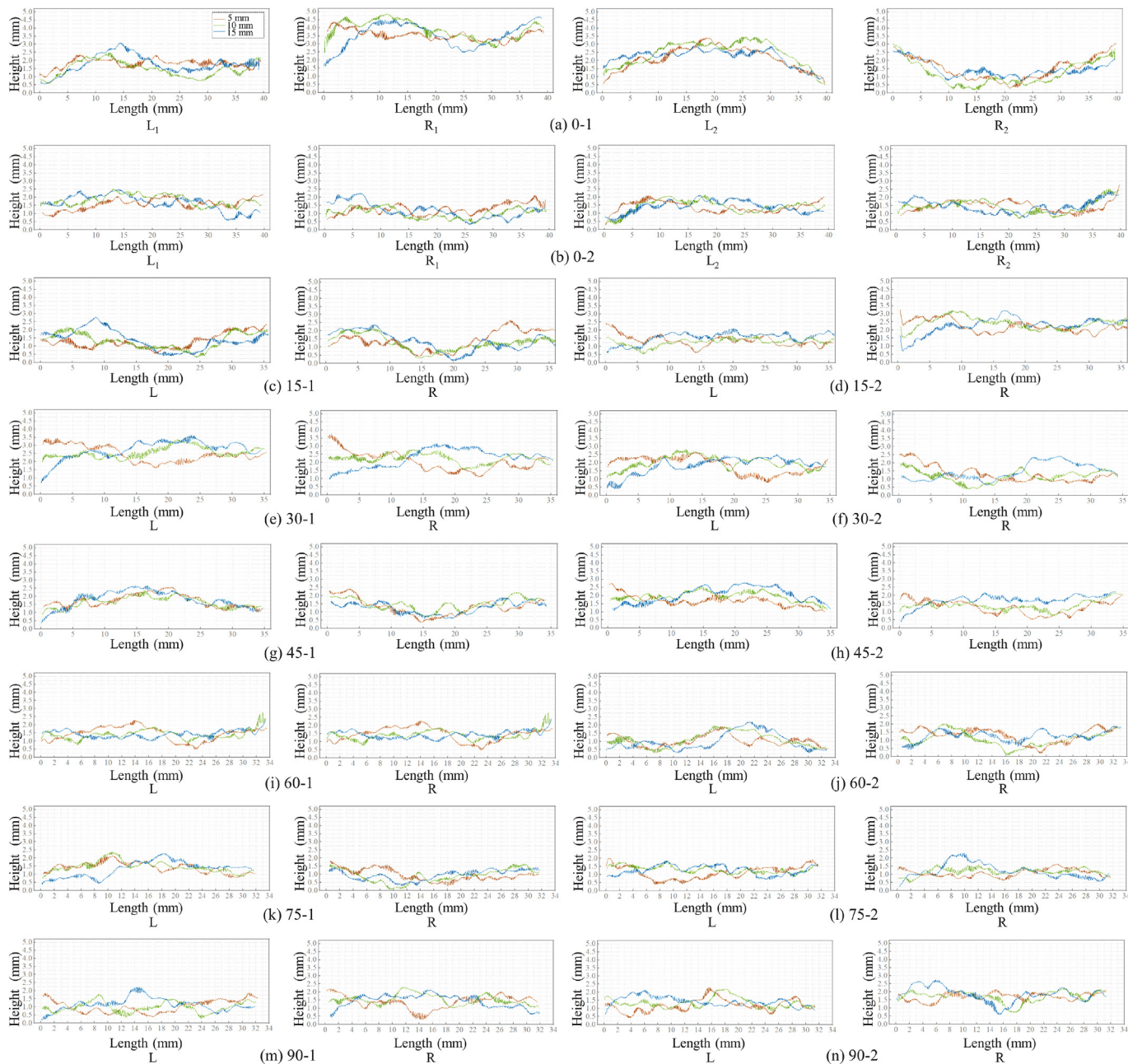
Fig. 8. 2D profiles of fracture surface at different locations.
