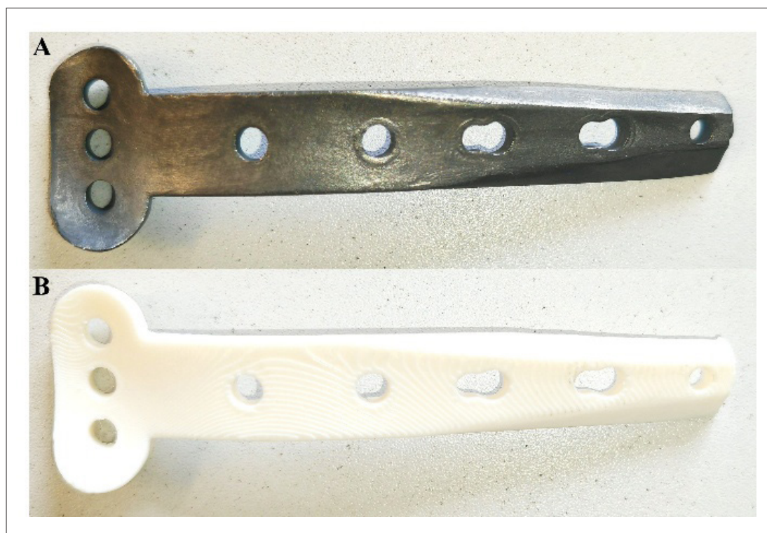
Figure 4. Fabricated generatively designed plates: (A) the metal generatively designed bone plate manufactured from Ti6Al4V via laser powder bed fusion after post-processing; (B) the corresponding poly(lactic acid) prototype fabricated by fused deposition modeling for early-stage biomechanical validation.
