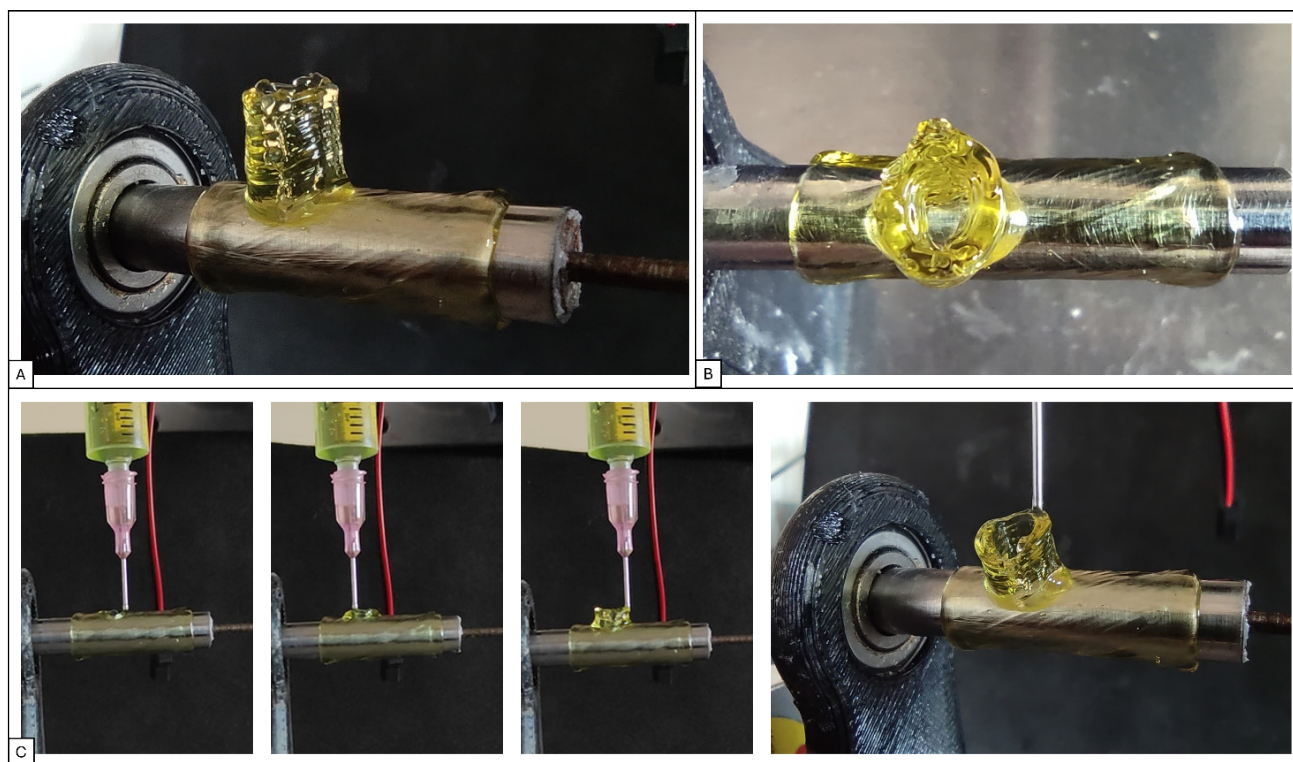
Figure 9. Cylindrical extrusion-based bioprinting printing results. (A) Final printed product. (B) The central channel of the lateral branch, demonstrating an open structure that maintains its integrity. (C) Printing process: after depositing the first cylindrical layers to create the main branch, the lateral branch is formed by depositing material layer by layer with an increasing radius. As it develops radially, no supports are required.
