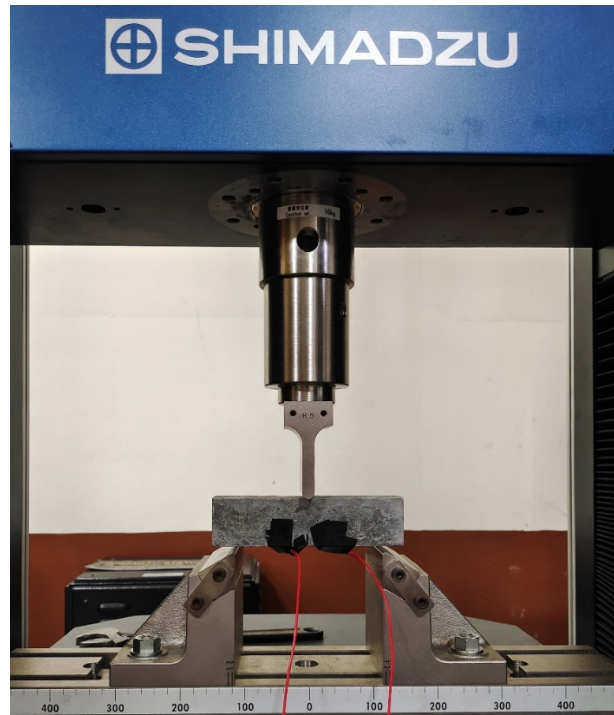
Fig. S1 An example of TPB test using SHIMADZU universal testing machine.
