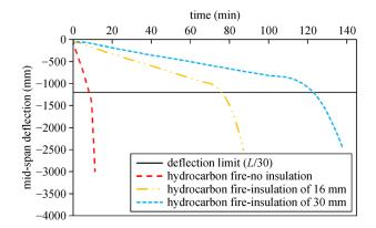
Fig. 6 Comparison between mid-span deflection in uninsulated and insulated I-65 Birmingham Bridge girder.
