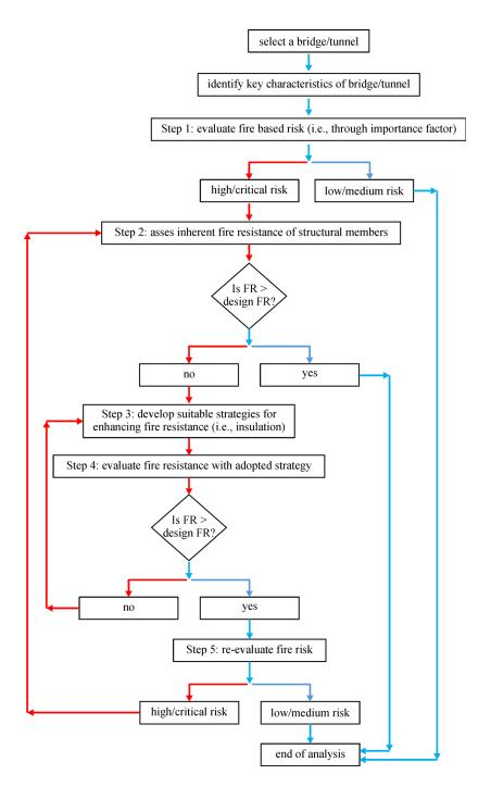
Fig. 2 Flow chart of the proposed approach for mitigating fire hazard in transportation structures (FR: Fire resistance).
