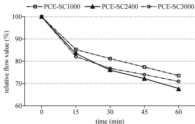
Fig. 2 Flow retention of mortar mixtures.
