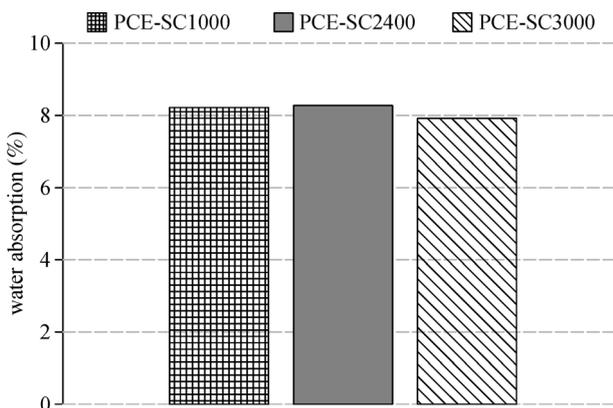
**Fig. 4** Water absorption of 28-d mortars containing HRWR admixtures
