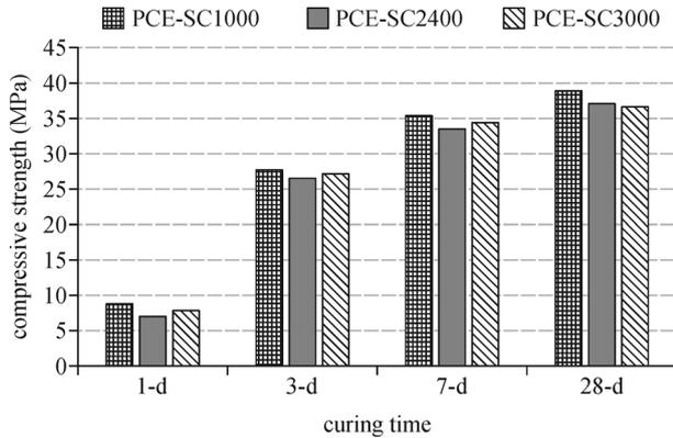
**Fig. 3** Compression strength of mortar mixtures containing HRWR admixtures.
