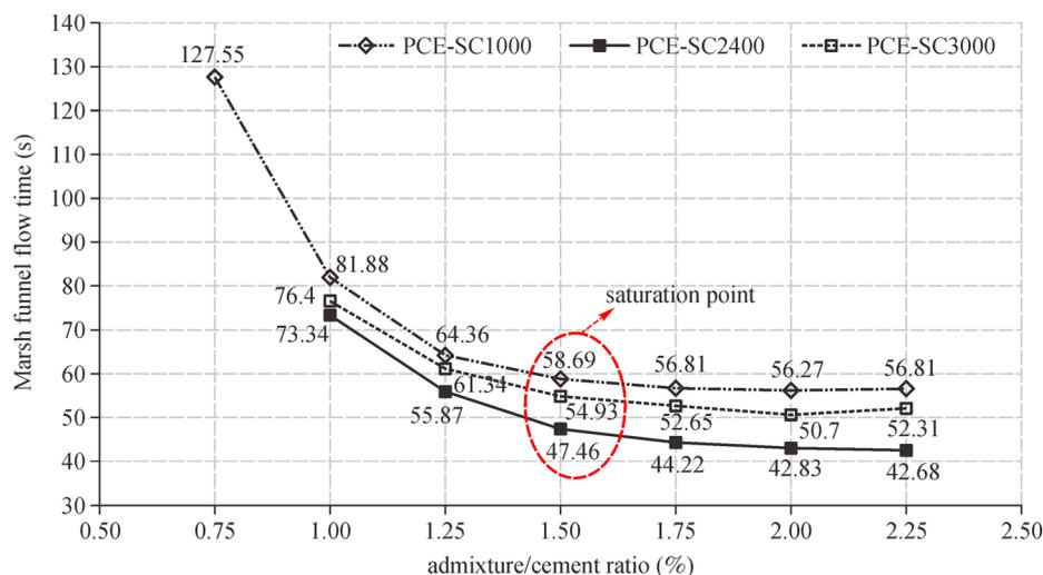
**Fig. 1** Marsh funnel flow times of cement pastes.
