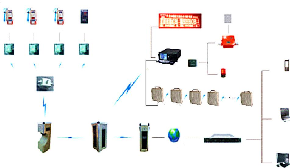
Fig. 4 Automatic wireless realtime gas monitoring system
