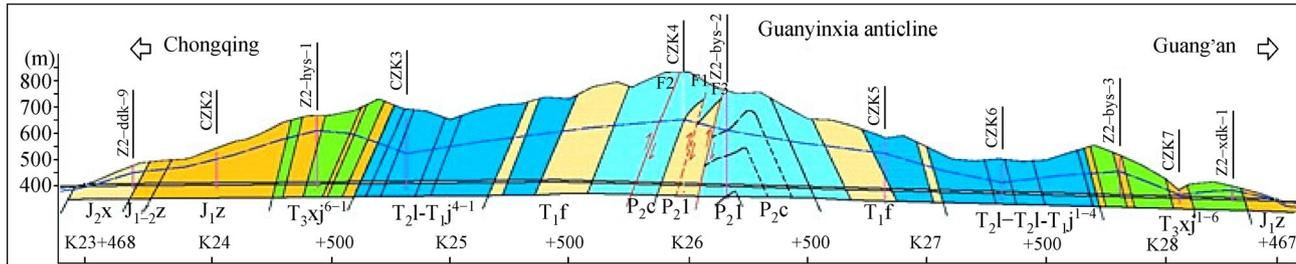
Fig. 2 Strata and tectonics of Huaying mount tunnel
