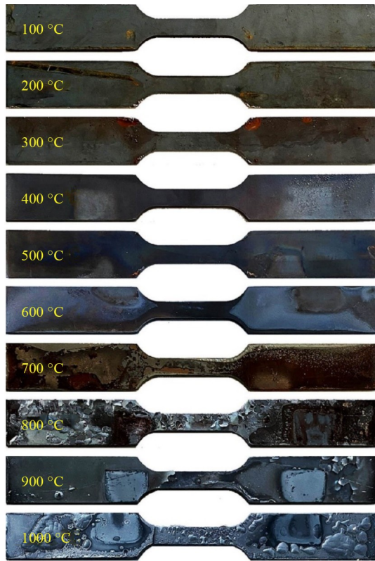
Fig. 11 Surface conditions of the tensile coupons prior to post-fire tests.
