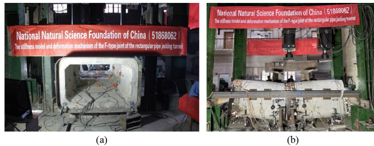
Fig. 2 Laboratory joint test: (a) laboratory joint shear test; (b) laboratory joint bending test.
