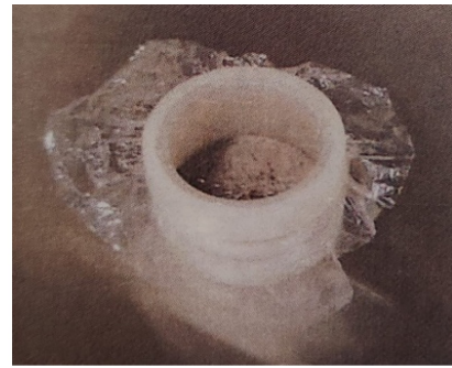
Fig. 11 FA sample placed in PP cap.
