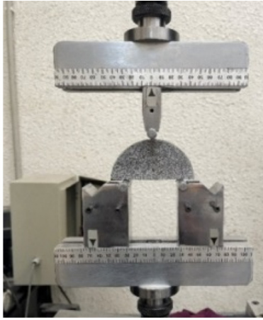
Fig. 4 Setup for three-point bending of SCBs.
