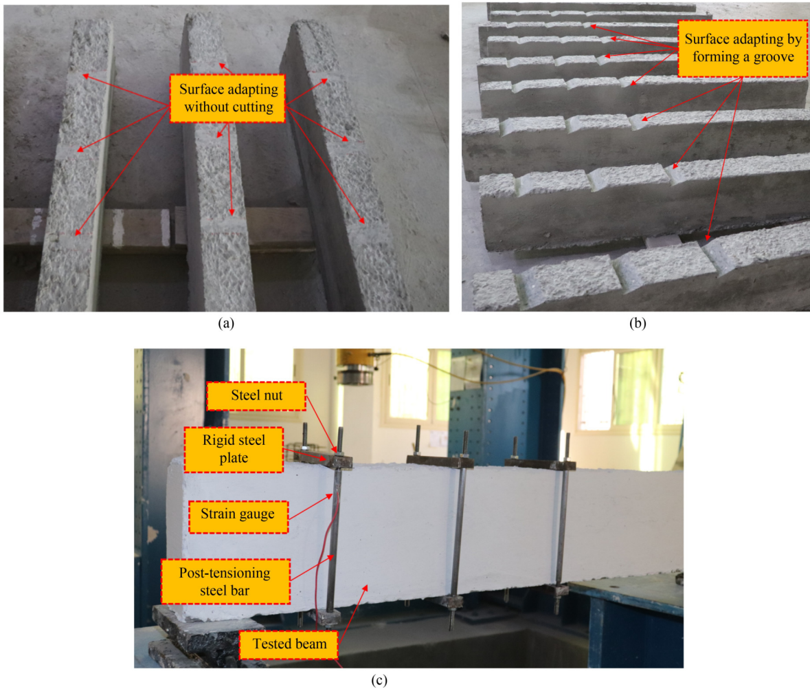
Fig. 7 Strengthening preparation: (a) vertical post-tensioning adapting; (b) inclined post-tensioning adapting; (c) applying post-tensioning force.
