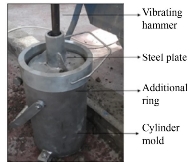
Fig. 2 Vibrating hammer, steel plate, additional ring, and cylinder mold used to produce RCC specimens.
