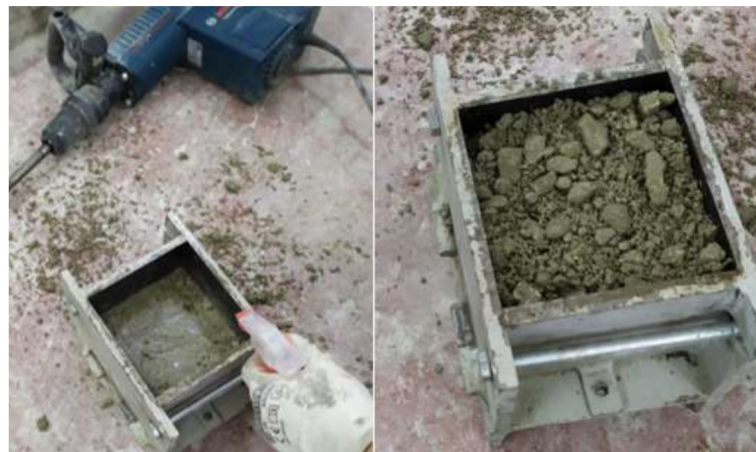
Fig. 6 Placement of cube specimens in molds.
