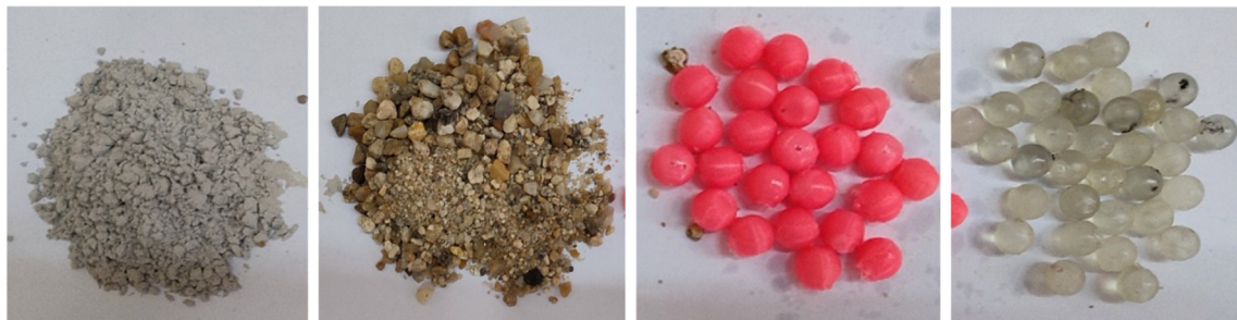
Fig. 2 From left to right, the appearances of GGBS sand 3D printed FDM aggregates and 3D printed SLA aggregates.
