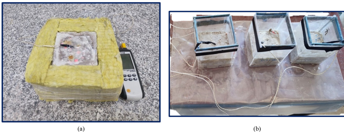
Fig. 5 (a) The thermal response of concrete surfaces; (b) the observation of ice formation on concrete surfaces.
