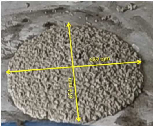
Fig. 1 Slump flow of the LWSCGC.
