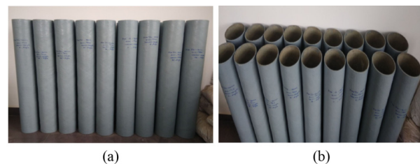
Fig. 2 GFRP tubes: (a) front view; (b) top view.
