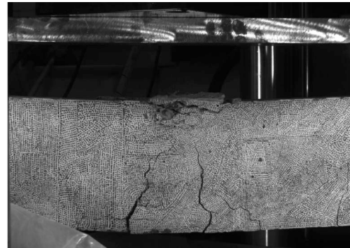
Fig. 11 Specimen complete failure.
