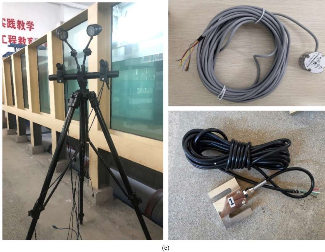
Fig. 1 Experimental setup of SFT model. (a) Mooring style 1; (b) mooring style 2; (c) mooring style 3; (d) schematic illustration of experimental setup; (e) main measuring equipment.
