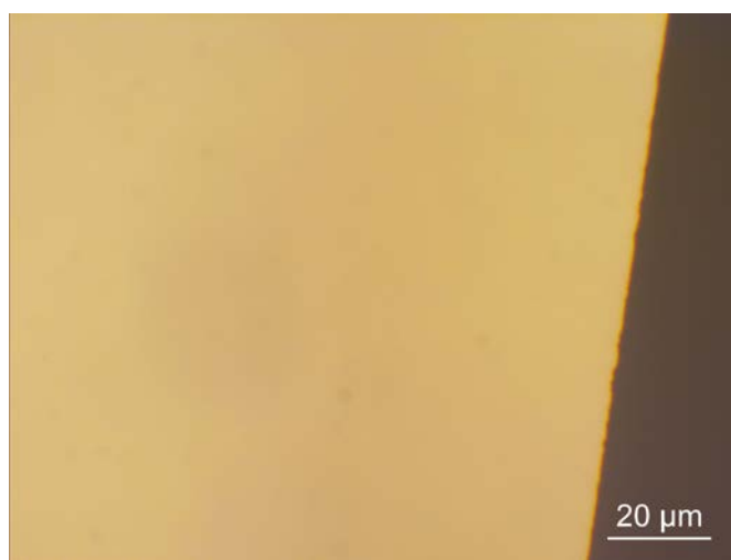
Fig. S1 Optical image of large-scale continuous silver flakes transferred on the polydimethylsiloxane (PDMS) substrate.
