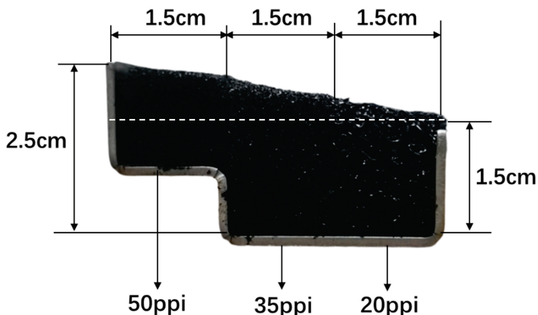
Fig. S7 Cross sectional view of the water elimination device. It is divided into three layers, and the pore size of the sponge increases from left to right [1].
